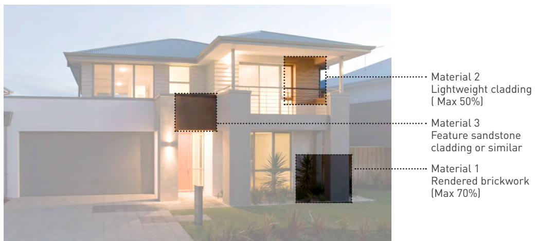
Figure 2 Example of appropriate mix and proportion of material
