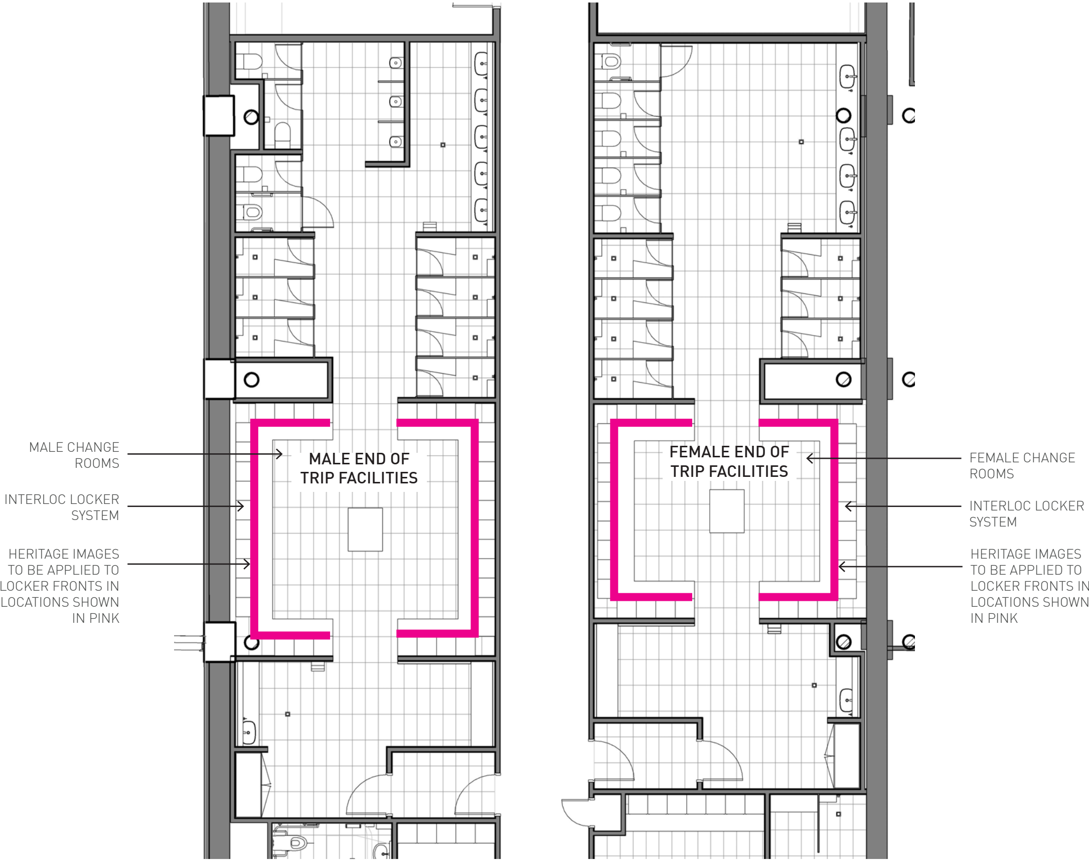
END OF TRIP FLOOR PLAN - LOCKER INTERPRETATION LOCATION
