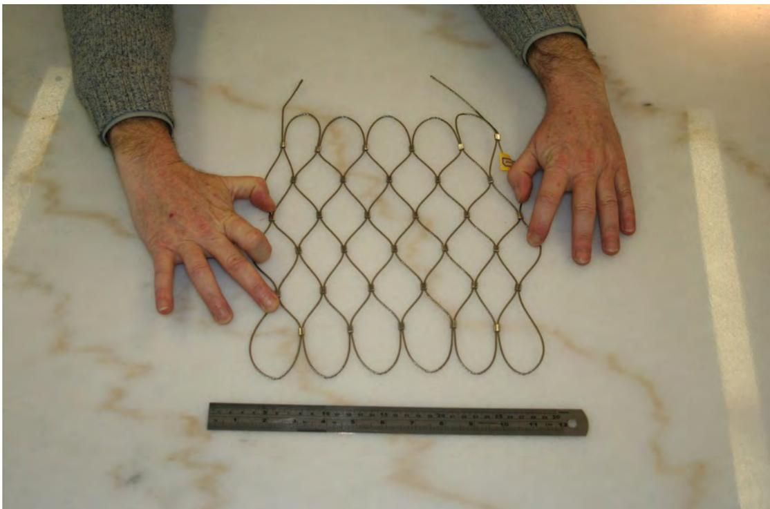
Figure 27 – RaMeiJu 60mm stainless steel mesh. This is a similar, but slightly less refined mesh than the Ronstan.
