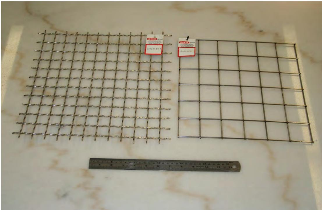
Figure 21 – Two examples of rigid stainless steel mesh, considered to be too bulky for screening use the context of the Boiler Area and Bay 1 Annex.
