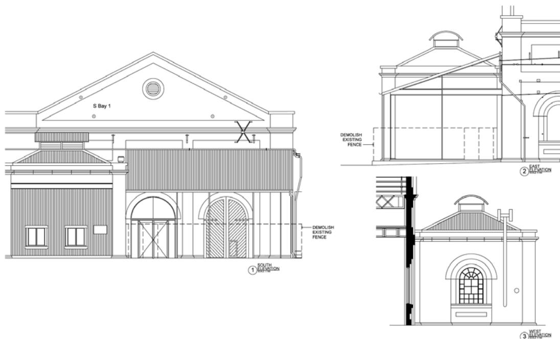
Figure 15 – The existing elevations of Bay 1 Annex.
