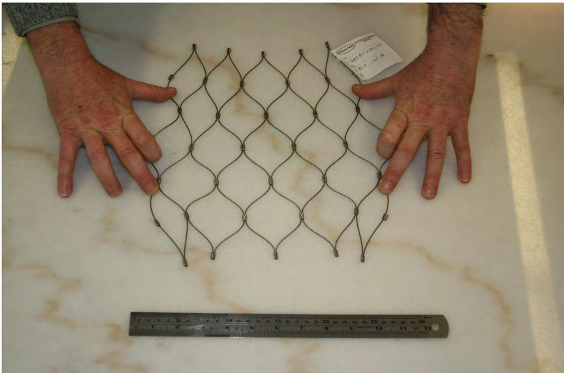
Figure 23 - Ronstan 60mm stainless steel mesh. A good mid-sized mesh.
