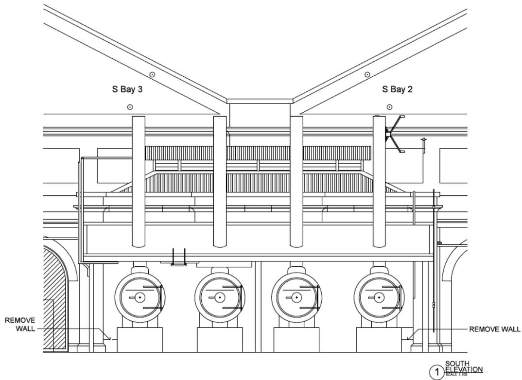
Figure 16 – The existing southern elevation of the Boiler Bay.
