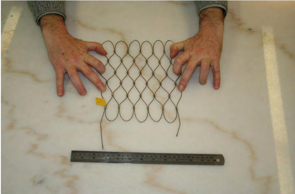
Figure 26 – RaMeiJu 40mm stainless steel mesh.
