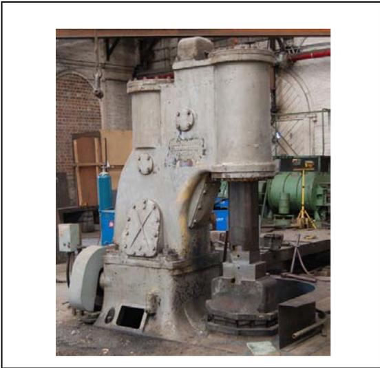
**Machine:** Massey 2CWT Weight Pneumatic Hammer
