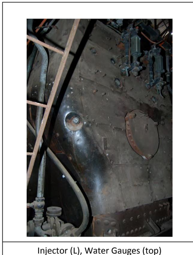
The level of water in the boiler is measured using the water gauge(s).
