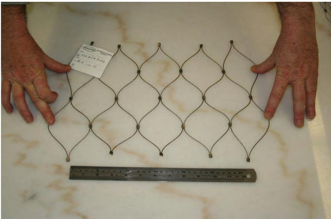
Figure 25 - Ronstan 80mm stainless steel mesh. This mesh is likely to be too open and may allow bird ingress.
