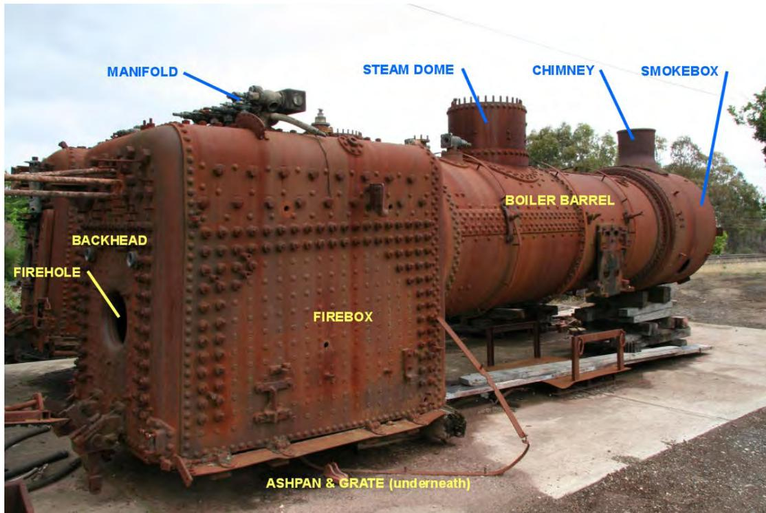
The diagram above gives a good insight into the main structural parts of a boiler similar to those existing at ATP. Because the ATP boilers were set up as stationary boilers, rather than being part of a moving locomotive, there are some significant differences to the normal layout. It is clear that changes have been made over time.
