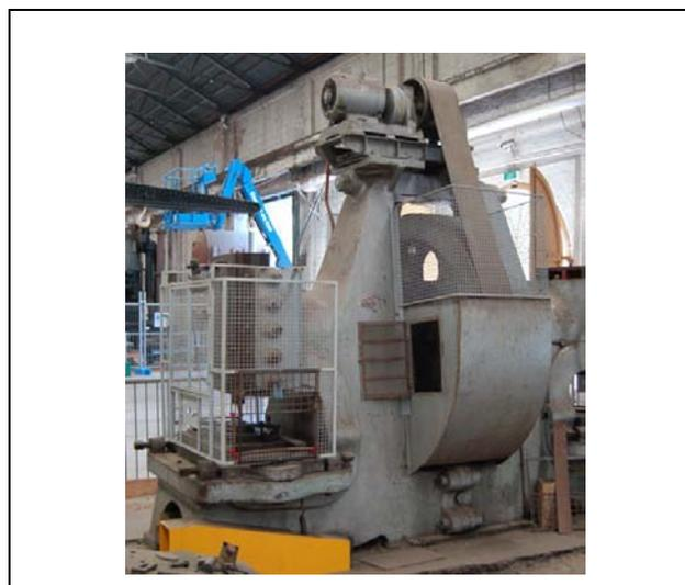
**Machine:** Massey 7CWT Electro-pneumatic Hammer
