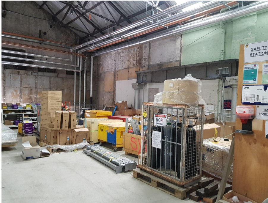
Photo 9: Inappropriate storage of gas cylinders near combustible materials
