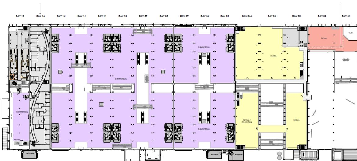
**Figure 14 Proposed Level 1 of the Locomotive Workshop**
